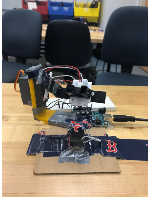
Figure 3: Our setup for both the one servo and two servo scan. We had to employ some creative, on-the-spot engineering to shift the sensor a little bit to be centered.
